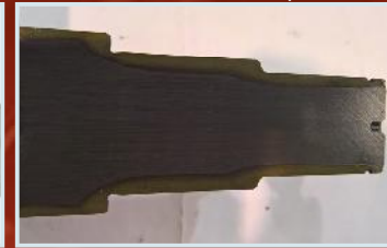
HIGH FREQUENCY Induction Hardening - Depth 1±4 mm
